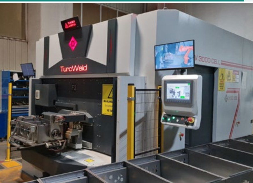
Robotic Laser Welding Machine for Wall Hung Boiler Body
