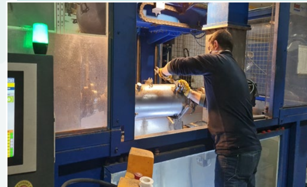
Boiler Air Testing System
