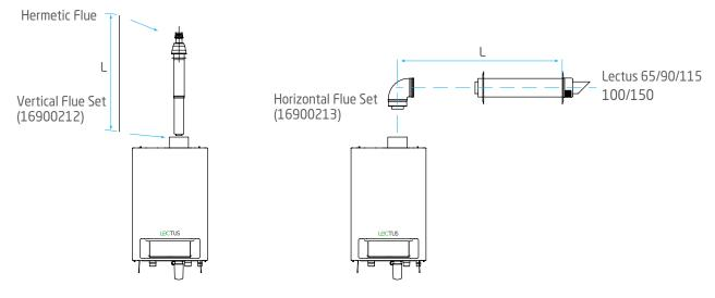
C13, C33, C43, C63, C93 flue types for hermetic arrangement.
